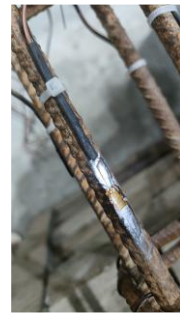
Step 4. Attaching the strain gauges (without any disturbance on the surface of gauges)
