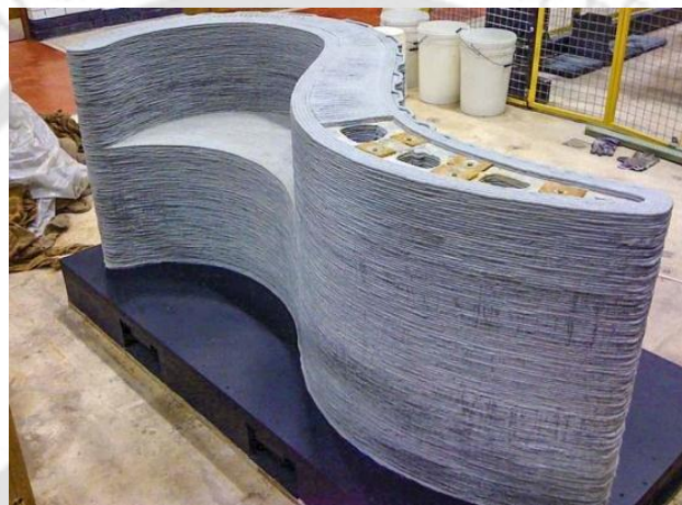
Fig. 2. 2 3D printed concrete bench [17].
