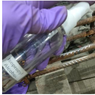
Step 2. Clearing the surface through Isopropyl spray to clear out the dust
