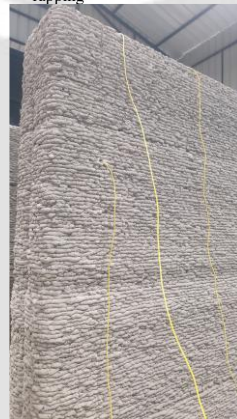
Step 11. A long wire (yellow) attached to strain gauges
