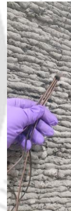
Step 11. Column insertion with attached strain gauges
