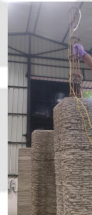
Step 11. Column insertion with attached strain gauges
