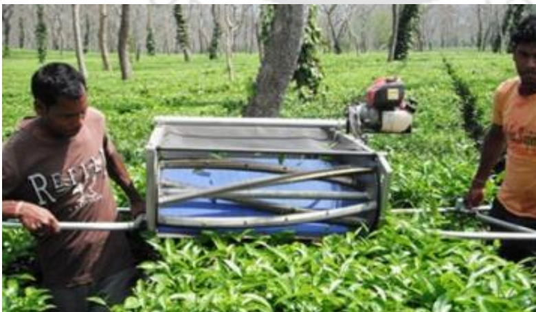
Fig. 4.4: Two persons, gasoline powered selective harvester. Source: Williame Tea
