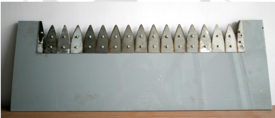
Fig. 5.21: Cutting blades attached on the base plate of the machine.
