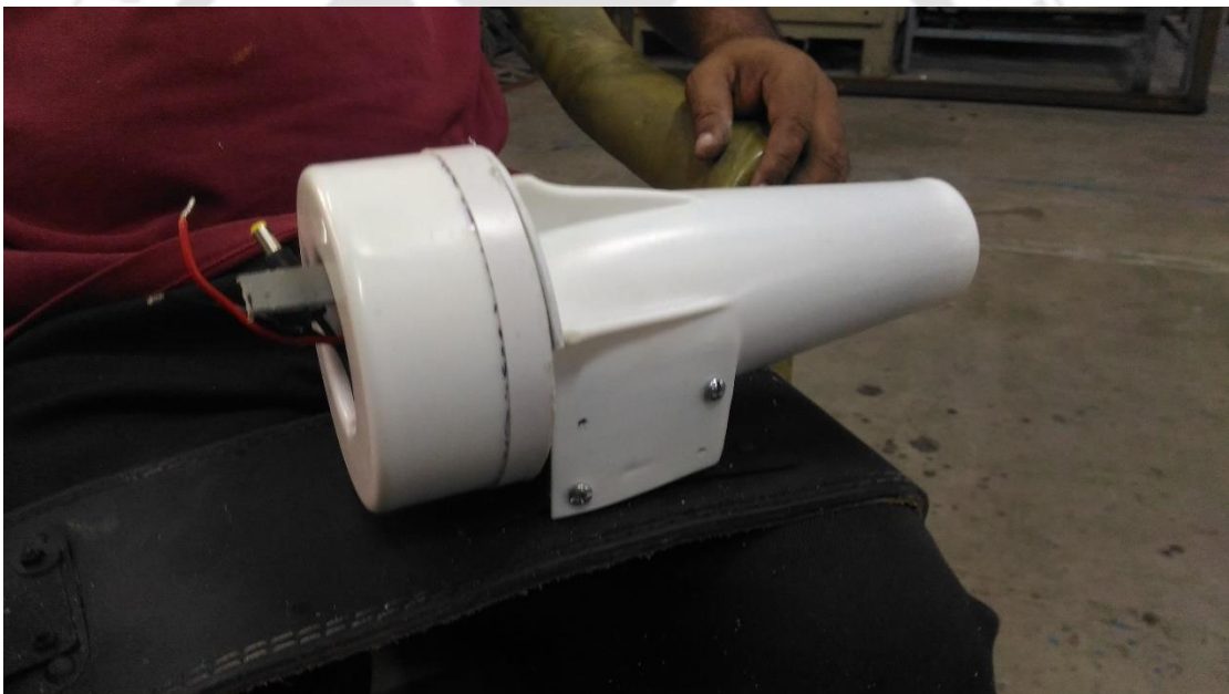
Fig. 5.30: Assembly of battery & prime mover module
