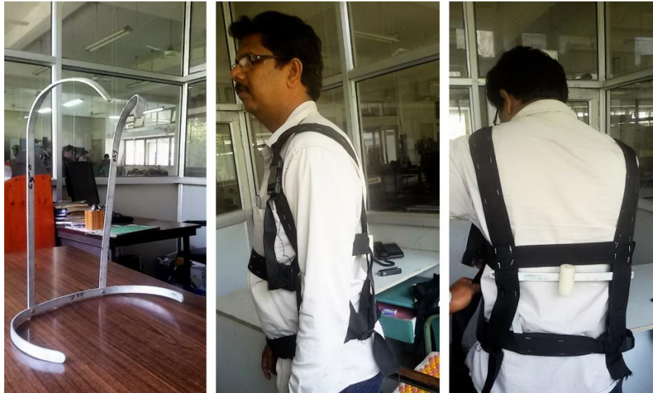
Fig. 5.42: Single lever mechanism with support from back strap
