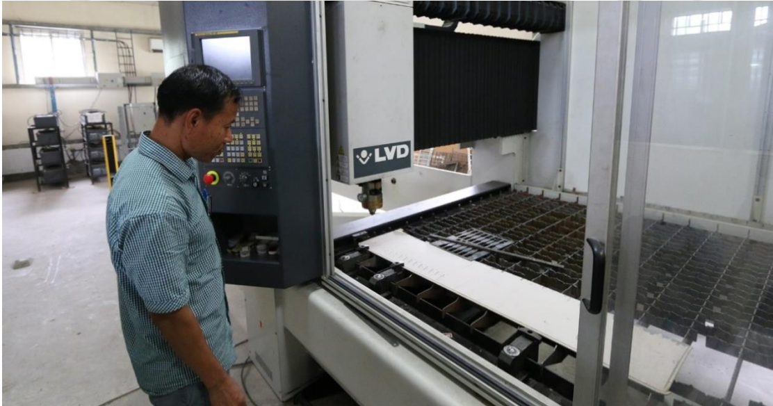
Fig. 5.18: Fabrication of stainless steel cutting blades with the help of Laser cutting machine.
