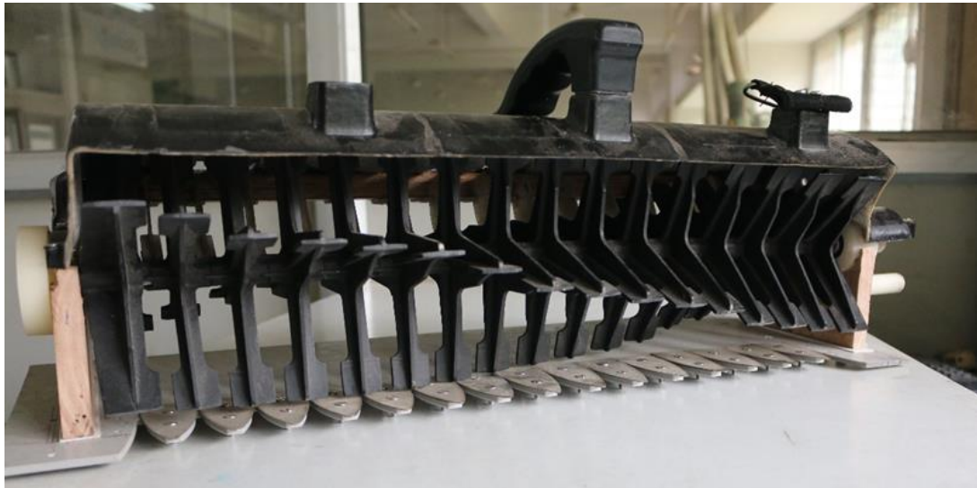
Fig. 5.26: Initial assembly of the machine showing rotor, cutting blades and spacers in casing
