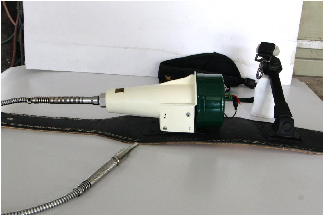
Fig. 5.31: Final assembly of battery module, prime mover module and attached with Bowden cable with waist belt
