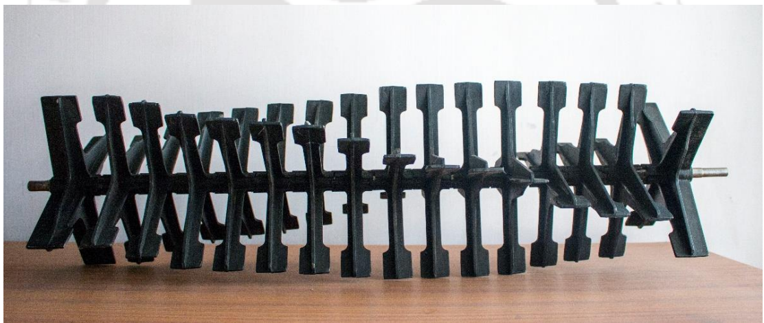
Fig. 5.16: Rotor & Driveshaft assembly after fabrication.
