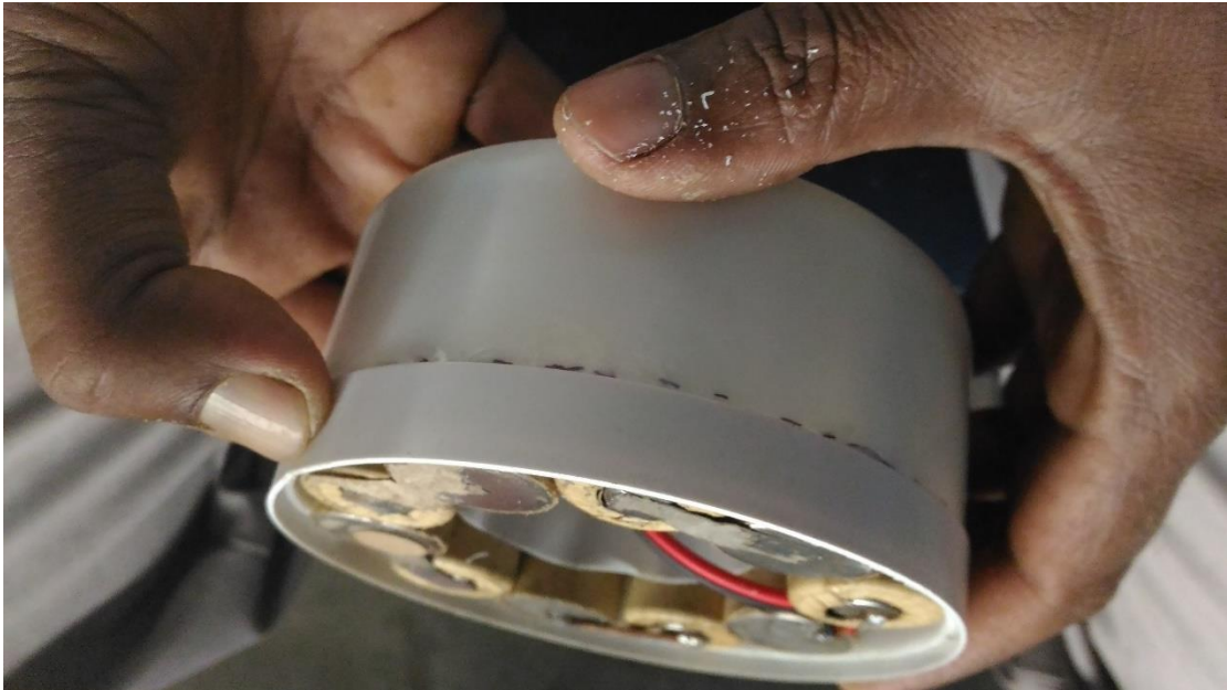
Fig. 5.29: Fabrication of battery cabinet
