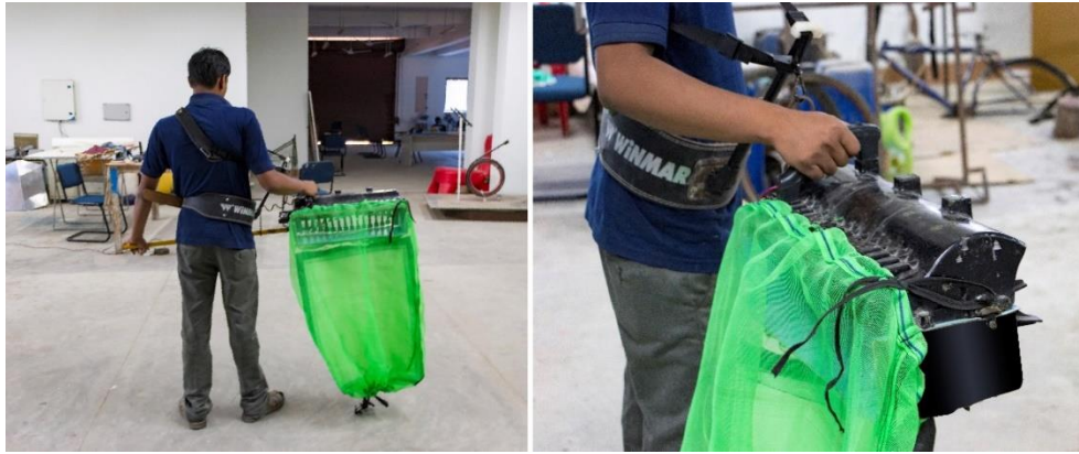
Fig. 5.35: Detachable type collection bag attached to the machine.
