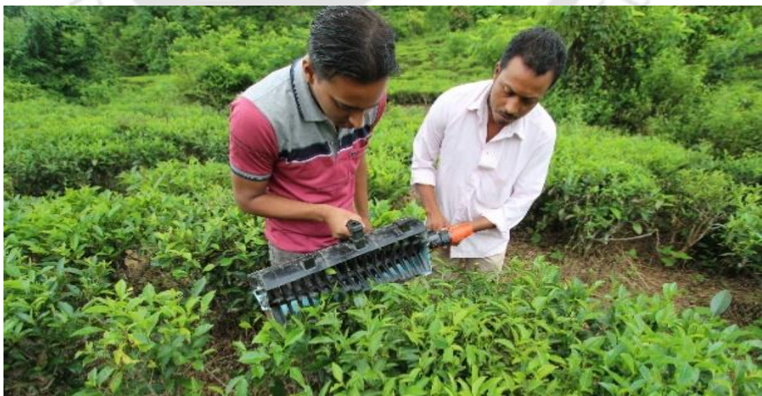
Fig. 5.50: Field experiment to find out the optimum revolution of the rotor shaft.
