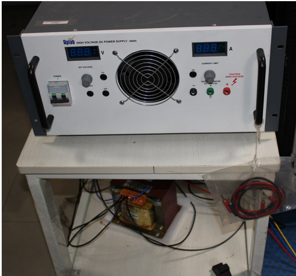
Fig. A.5 High voltage DC power source used to realize DG.
