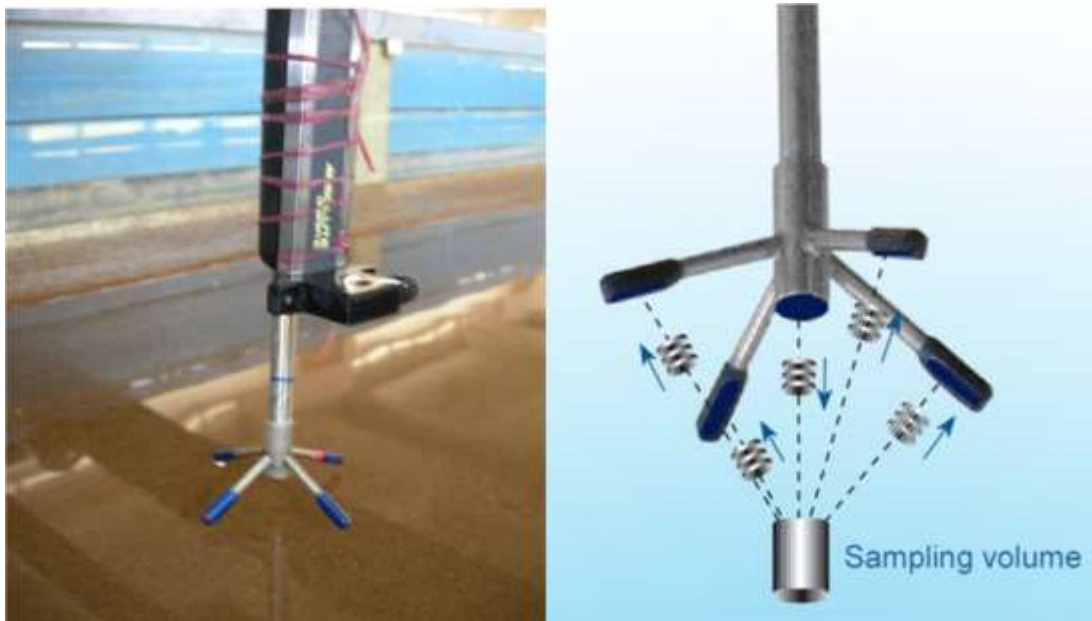
Figure 2.8 Acoustic Doppler Velocimeter for measuring instantaneous velocities
