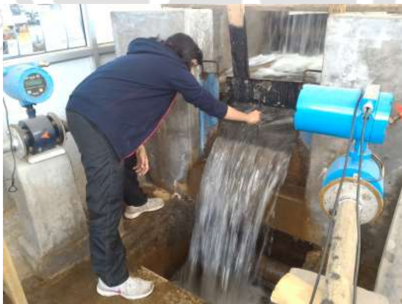
Figure 2.5 Measurement of main channel flow discharge over rectangular notch
