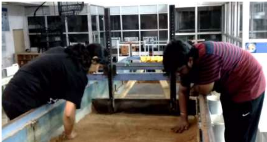
Figure 2.13 Bed preparation before installation of pier
