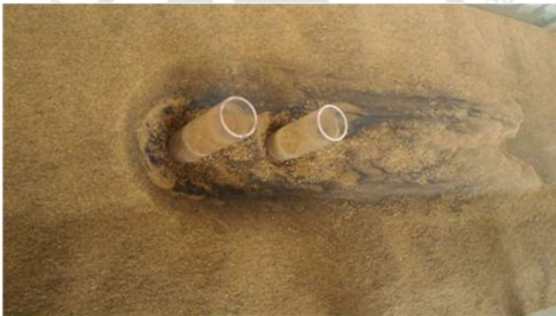
Figure 5.12 Snapshot of channel bed after scouring
