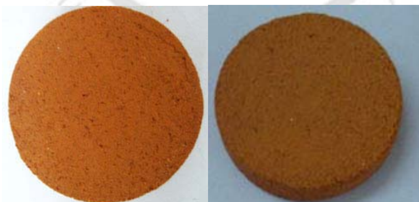
Fig. 3.8. Circular porous disk (CPD) made of red soil with 1 cm depth and approx 4.2cm diameter.
