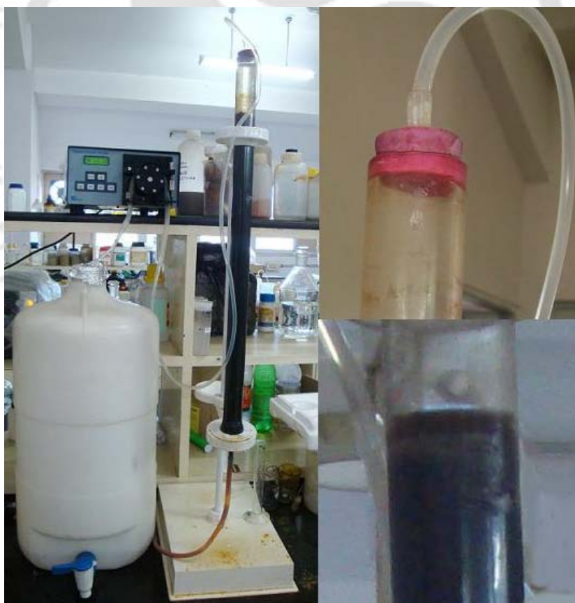
Fig. 3.7. Column experimental setup for NOIS adsorbent (Flow rate: 10 \text{ ml min}^{-1} , Bed depth: 45 cm).
