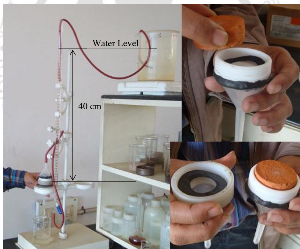
Fig. 3.9. Performance testing of the circular porous disk (water head= 40 cm).
