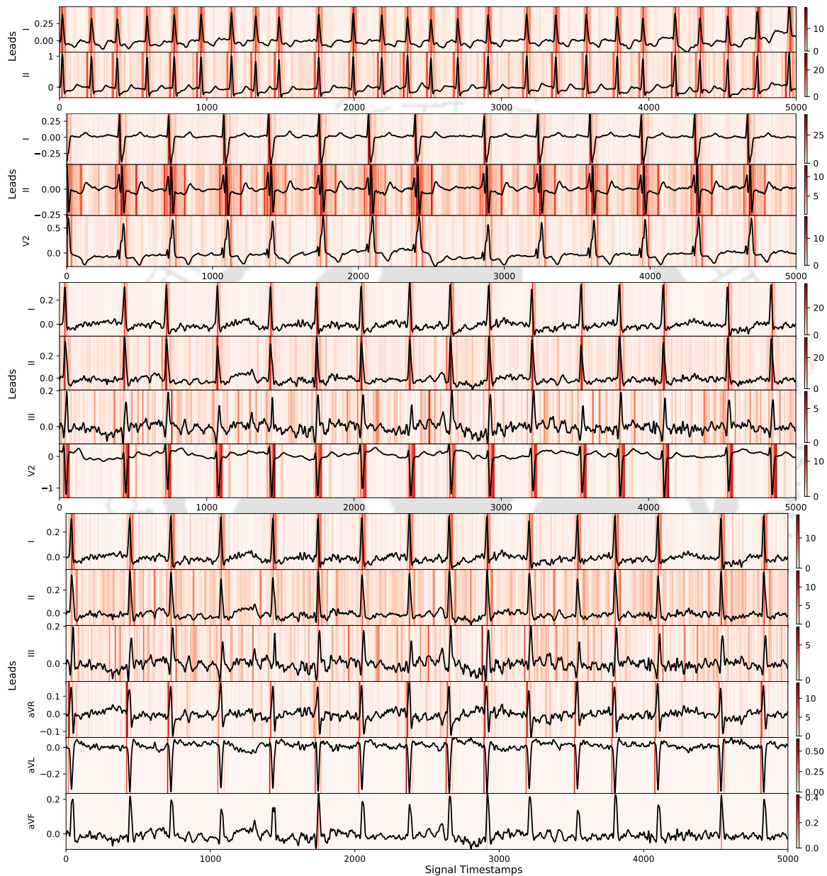
Figure 7.23: Signal contribution in each lead for multichannel ECG for AF pathology for different lead configurations. (Top to Bottom: Two, Three, Four, and Six lead). The attribution scores for each signal timestamp are represented with the amount of red colour assigned to the timestamp.
