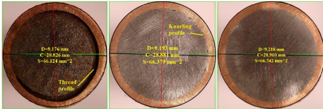
Fig. 4.13 Digital microscope images of the cross-section of the composite rods with measured outer diameter with (a) threaded, (b) knurled, and (c) plain profile at 5.3 kJ
