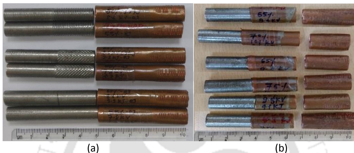
Fig. 4.8 Samples after pull-out test (a) failure in the joint at lower energy (2.7 kJ and 3.3 kJ), (b) failure in the tube at higher energy (3.9 kJ and 4.6 kJ)
