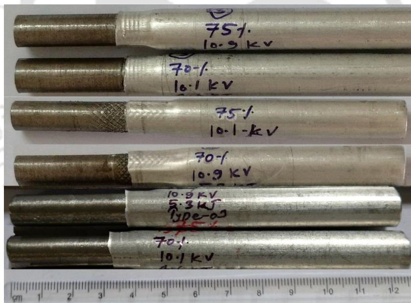
Fig. 5.6 Electromagnetic crimped samples with (a) threaded profile, (b) knurled profile, and (c) plain profiles on the base
