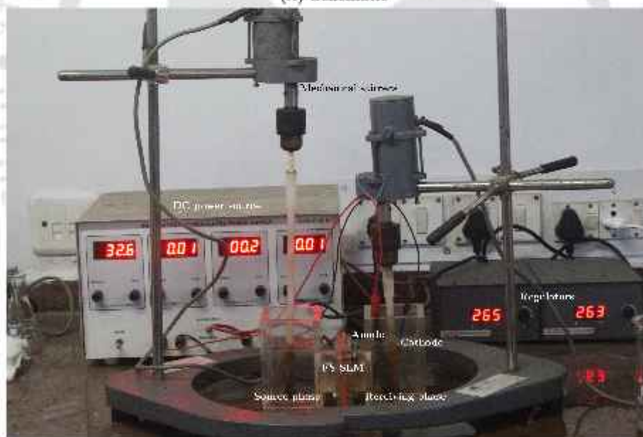
FIGURE 3.2: Experimental setup for three-phase FSSLM and hybrid technique
