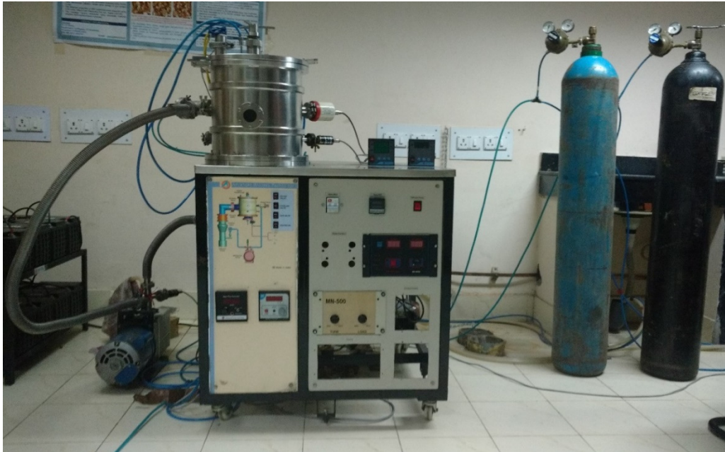
Figure 2.5 : Photographic view of the RF magnetron sputtering system.
