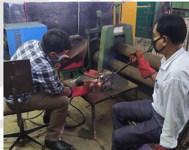
Joining cutter at base of fruit grabber
