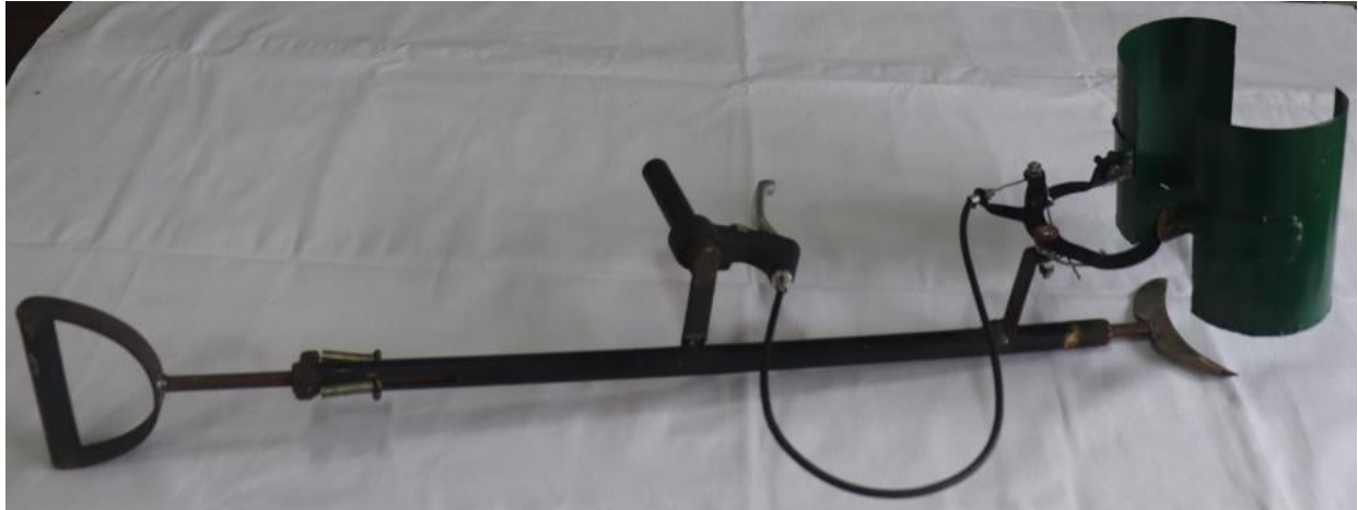
Figure 5.8. Prototype of manual pineapple harvester (Concept 3)
