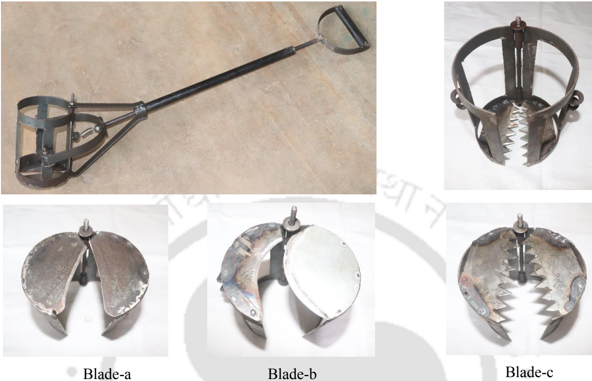
Figure 5.9. Prototype of pineapple harvester (Concept 4) with three designs of blade (a, b and c)
