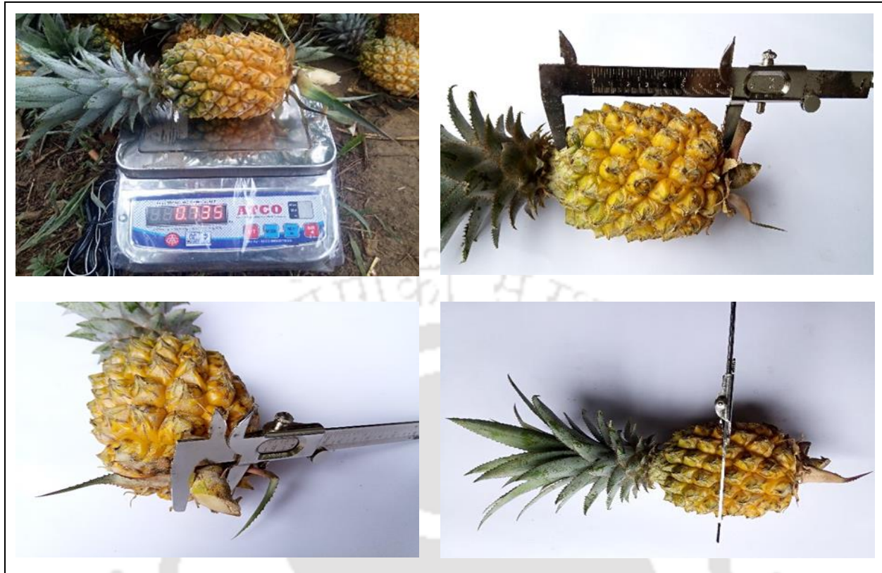
Figure 5.2. Measurement of physical properties of pineapple
