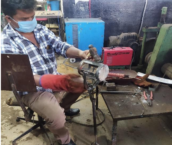
Adjustment of Flexible clamp attached with fruit grabber and handle
