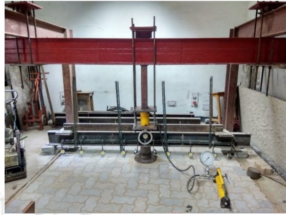
Figure 3.22: Plate load test on ICBP
