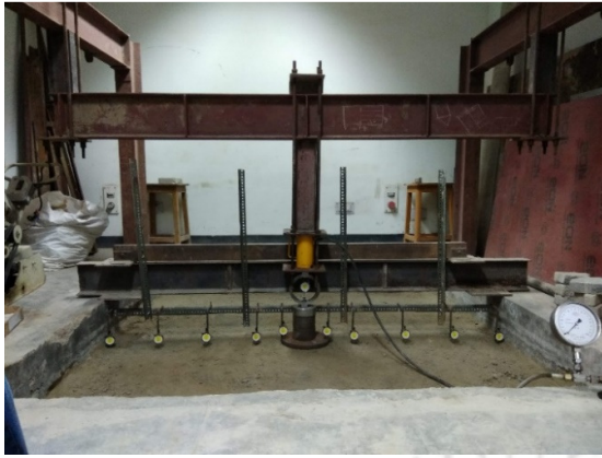
Figure 3.21: Plate load test on a granular layer
