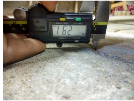
Figure 3.18: Joint width measurement
