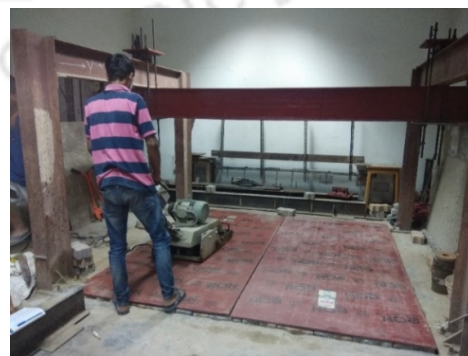
Figure 3.16: Compaction on ICBP
