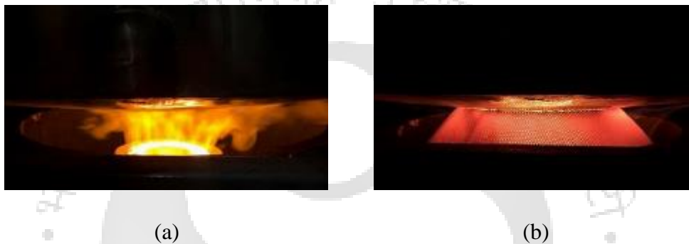
Fig. 2.7: Flames: APMB impinging flame (a) without PRRH and (b) with PRRH, Chaelek et al. (2019).
