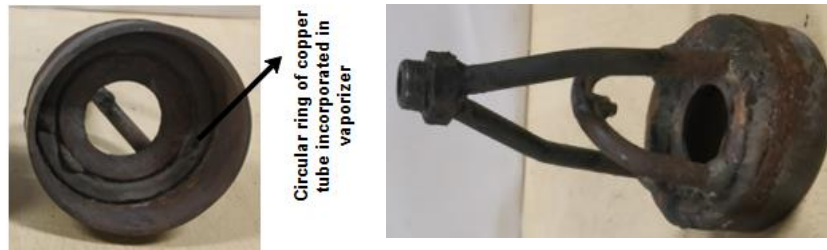
Fig. 6.5: Newly developed PRB for WCO and kerosene blend application.
