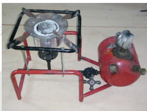
Fig. 6.3: Kerosene operated PRB developed by Sinha, 2017.
