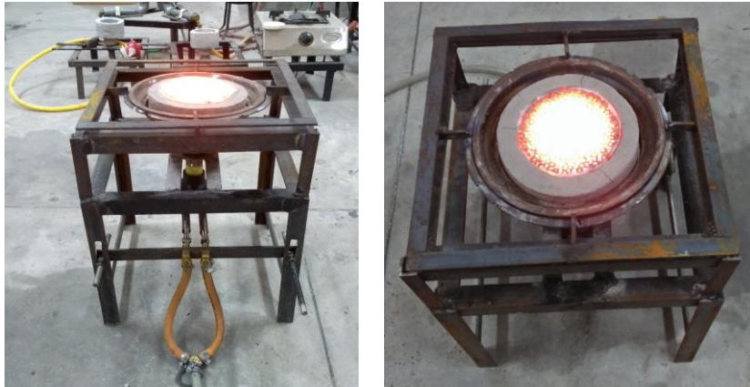
Fig. 4.6: Pictorial view of the LPG operated PRB cook stove (5-7 kW) in running condition.
