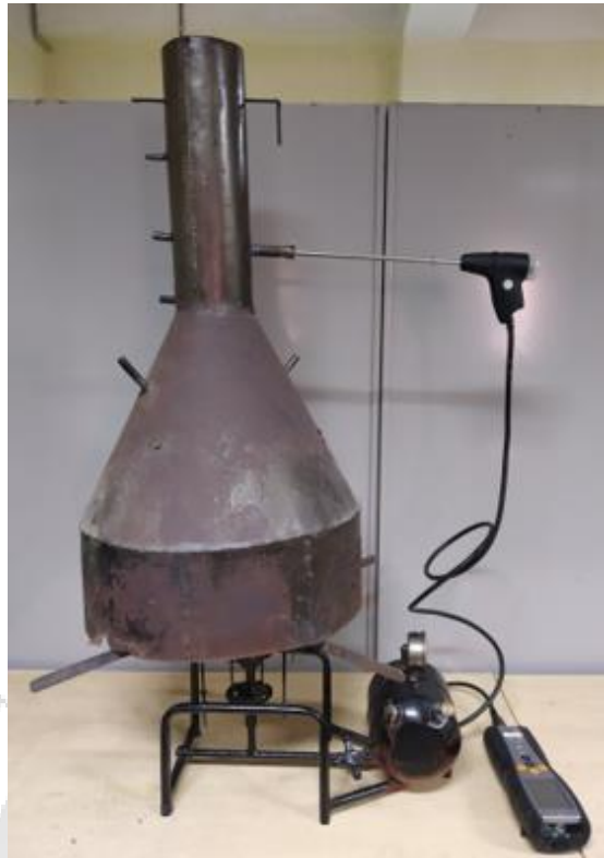
Fig. 6.22: Photographic view of experimental setup for measuring emissions.
