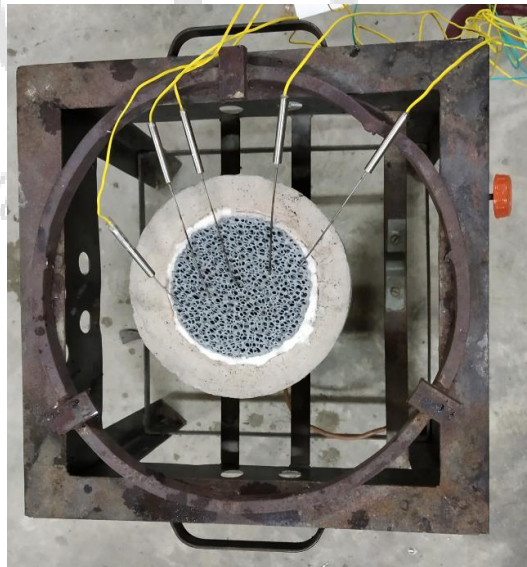
Fig. 4.9: Photographic view of thermocouple over self-aspirated PRB surface (5-7 kW).
