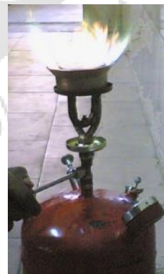
Fig. 2.25: Oil stove developed by Natarajan et al. (2008).
