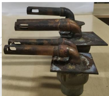
Fig 4.4: Different burner ports (Dia. 15.8 mm, 19 mm and 21 mm ) with connector used in the present work.
