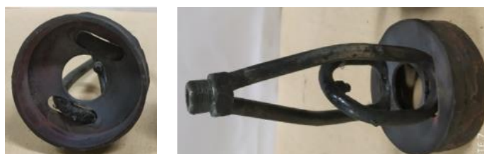
Fig. 6.4: PRB assisted kerosene vaporizer developed by Sinha, 2017.
