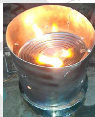
Fig. 2.28: Modified pressurized cooking stove, Suhartono et al. (2017a, 2017b).
