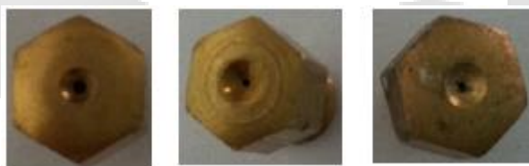
Fig. 4.5: Orifices of 0.25 mm,0.35 mm,0.5 mm and 0.8 mm diameters.
