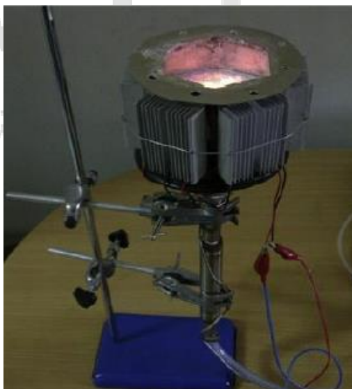
Fig. 2.9: The micro-cogeneration system developed by Ismail et al. (2013).
