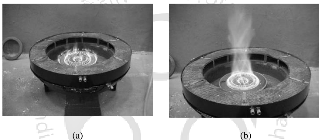
Fig. 2.3: (a) Conventional radial flow flame (CB) and (b) Swirling central flame (SB) in the PRRB housing, developed by Jugjai and Rungsimuntuchart (2002).
