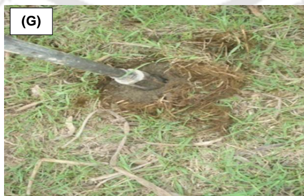
Figure 2.3 (G) Soil sampling with an auger at different depths in Majuli River Island
