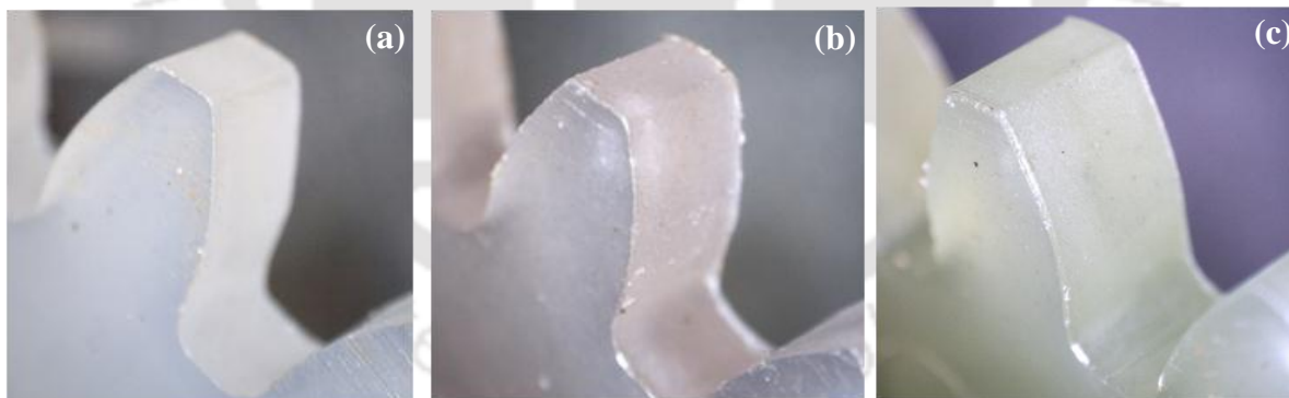
Figure 6.12: Tooth surface of prepared gear (a) pristine PS, (b) PSCL 1 and (c) PSNL 1 nanocomposites.
