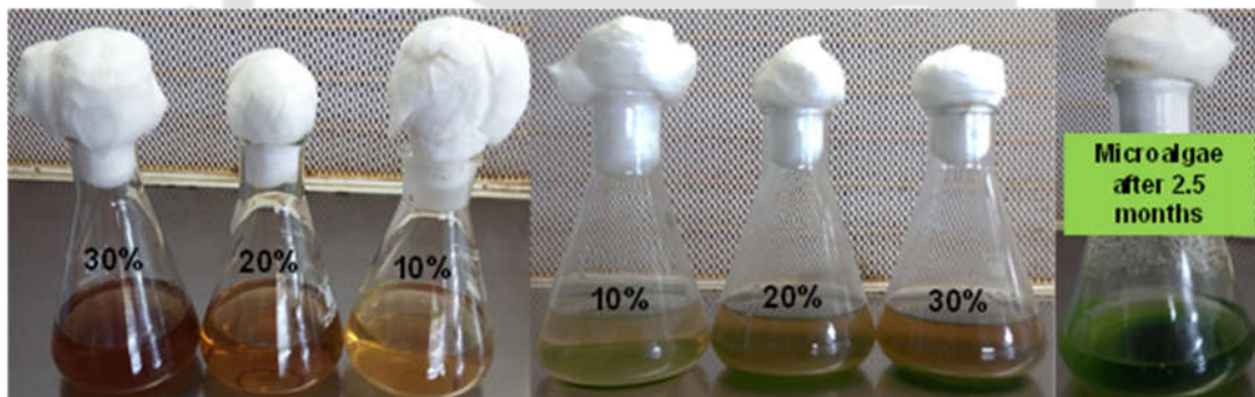
Figure 7.2: Growth of microalgae under different dilution of biogas plant digestate.
