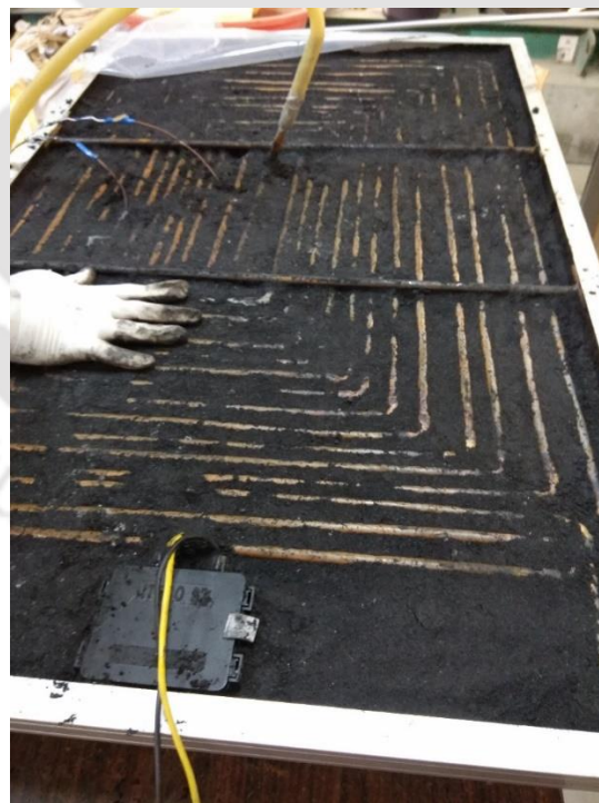
Figure IV.4. PV/T collector with novel PCM-biochar composite
