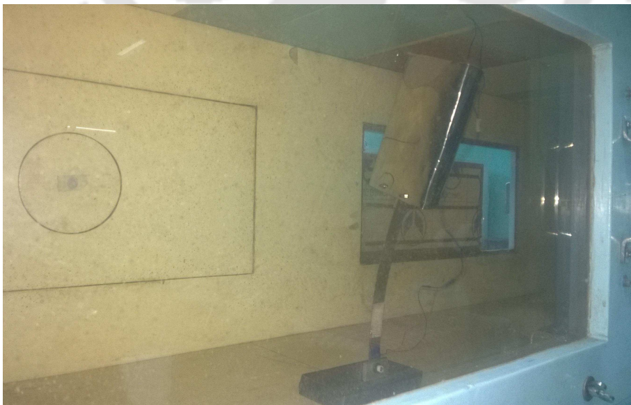
FIGURE 6.7: Galloping of GPEH system inside the wind tunnel
