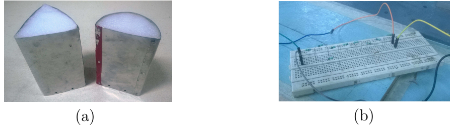
FIGURE 6.8: (a) D and Triangular shape bluff bodies (b) External electric circuit with load resistances
