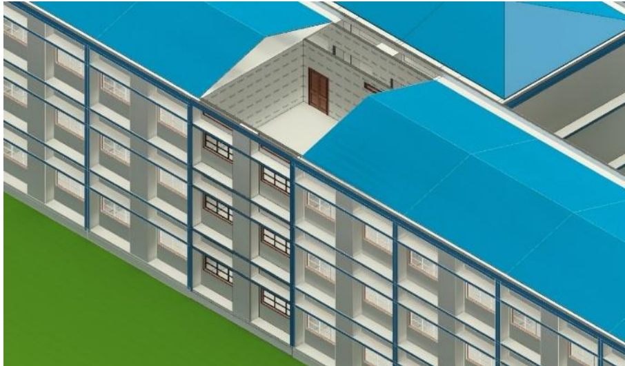
Figure 46: 3D view of the base-case classrooms with PCM added in all walls and ceilings.
