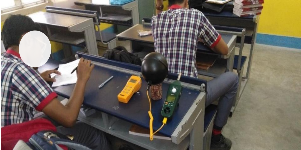
Figure 7: Extech-5 in 1 Environment Meter along with globe thermometer and CO 2 meter
