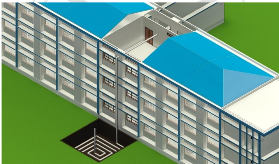
Figure 47: 3D view of the base-case classrooms with EAHE installed in the classrooms.
