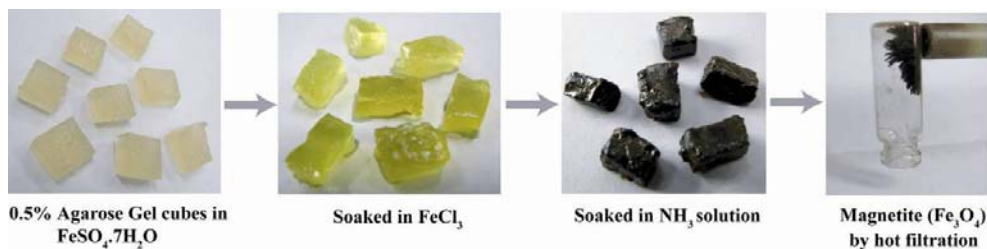
Scheme 4.6. Magnetite synthesis in 0.5% Agarose Gel.
