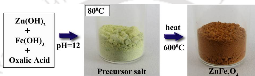
Scheme 4.4. Synthesis of Zinc ferrites by thermolysis of Zn(II)-oxalic acid precursor salts.
