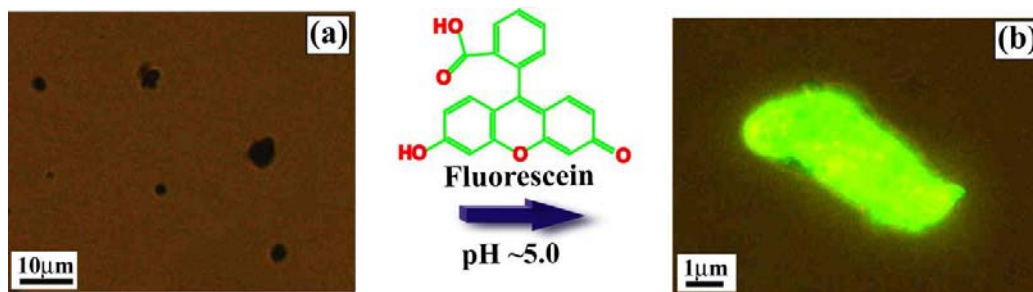
Figure 4.22. Fluorescence optical microscope image of magnetite particles (a) before and (b) after fluorescein adsorption.
