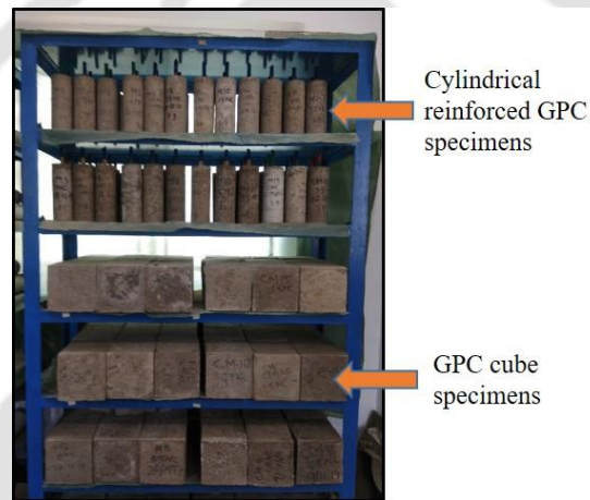
Fig. 3.14 Photograph of cubes and cylindrical reinforced specimens prepared in 2 nd phase of experiment of GPC series.
