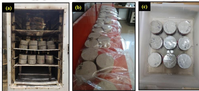
Fig. 3.8 Photographs during (a) oven drying, (b) pre-conditioning, and (c) sorptivity test of GPM specimens.
