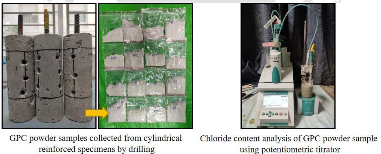
Fig. 3.17 Photographs of drilled cylindrical reinforced specimens, GPC powder samples, and chloride analysis using potentiometric titrator.
