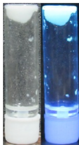
Figure 4.15. Photograph of the gel after keeping inverted for 25 days showing the formation of xerogel under daylight and UV light ( \lambda_{\text{max}} = 365 \text{ nm} )
