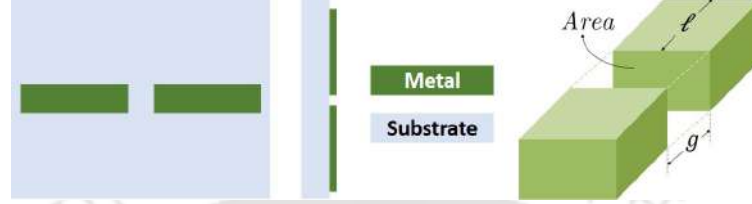
Figure 2.7: Illustration of capacitance formation and inductance between two conducting strips.
