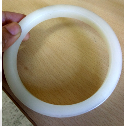
Figure 3.5: Nylon ring made to be placed upon the master.
