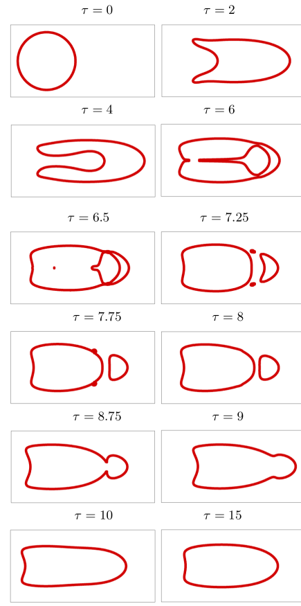
Figure 4.11: The shape evolution of a droplet for Ca = 1 and \lambda = 0.1 . The aspect ratio a = 0.8 .
