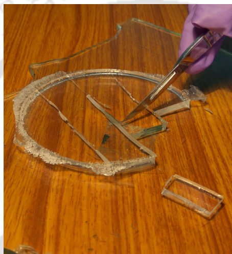
Figure 3.7: Cutting the solidified PDMS to make channels.
