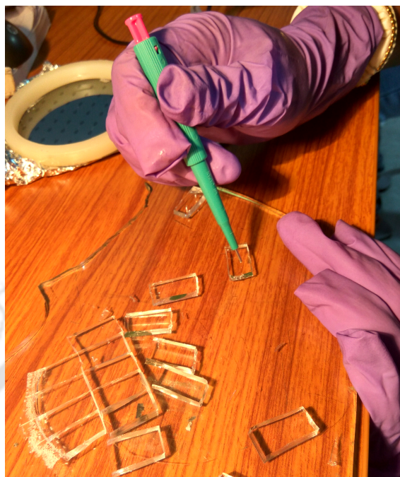
Figure 3.9: Thorough holes for inlet and outlet are punched with the help of punching tool.
