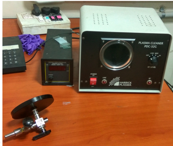
Figure 3.11: An image of the oxygen plasma chamber.
