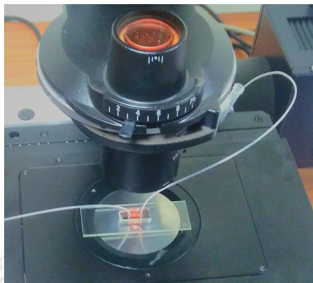
Figure 3.14: A magnified image of the channel placed on the stage of the microchannel with connecting tubes inserted at the inlet and the outlet.
