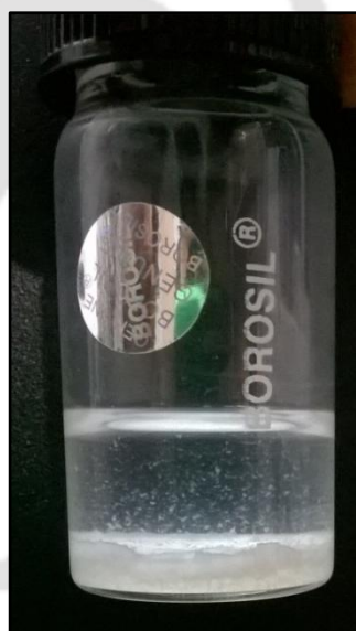
[D] Settling down of the precipitate to the bottom
