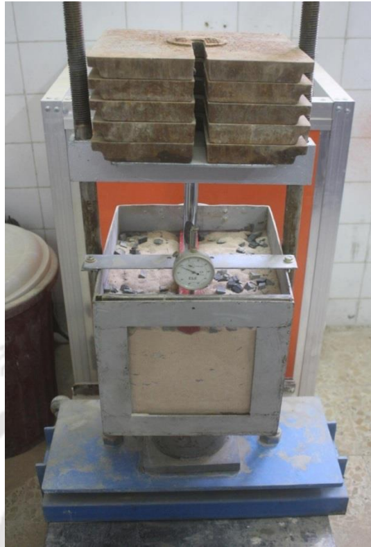
Fig. 2.27 Model container for typical foundation (after Alqaissi 2012)
