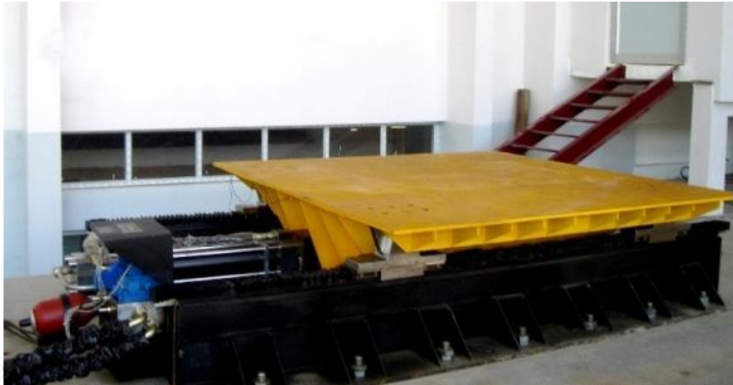
Fig. 3.16 Shaking table at IITGuwahati
