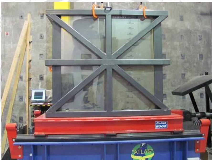
Fig. 2.10 Shake table test of seismic responses of MSE walls (after Xiao et al. 2012)
