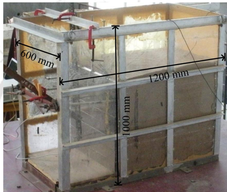
Fig. 3.19 Typical model wall with container
