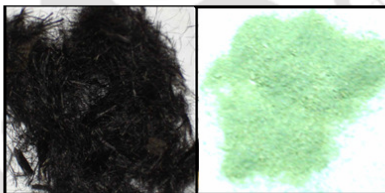
Figure 4.43 (a): Cr(VI) contaminated PANI-jute and Figure 4.43(b) Oxides of chromium after ignition of Cr(VI) contaminated PANI-jute
