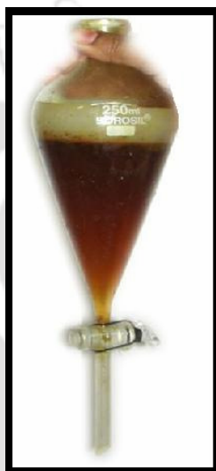
Figure 3.3: Separation of chloroform-AFC resin mixture from aqueous solution
