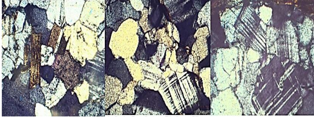
Figure 68. Thin-section microscopic images of porphyritic granite showing the presence of biotite and microcline deformed plagioclase feldspar with large Quartz grains in the stone sample KMT-01 SDT-01 and KMT-03 KDT-01.
