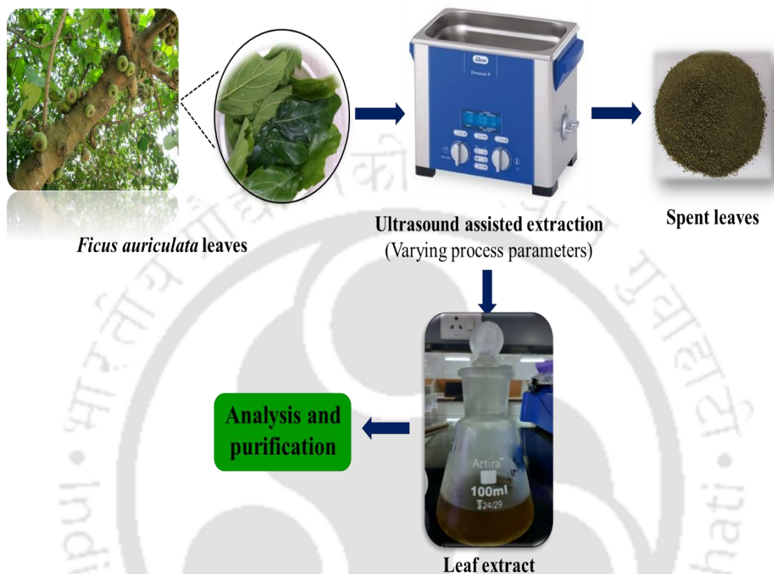
Figure 2.1 Ultrasound – assisted extraction process of gallic acid from F. auriculata leaves at 37 kHz
