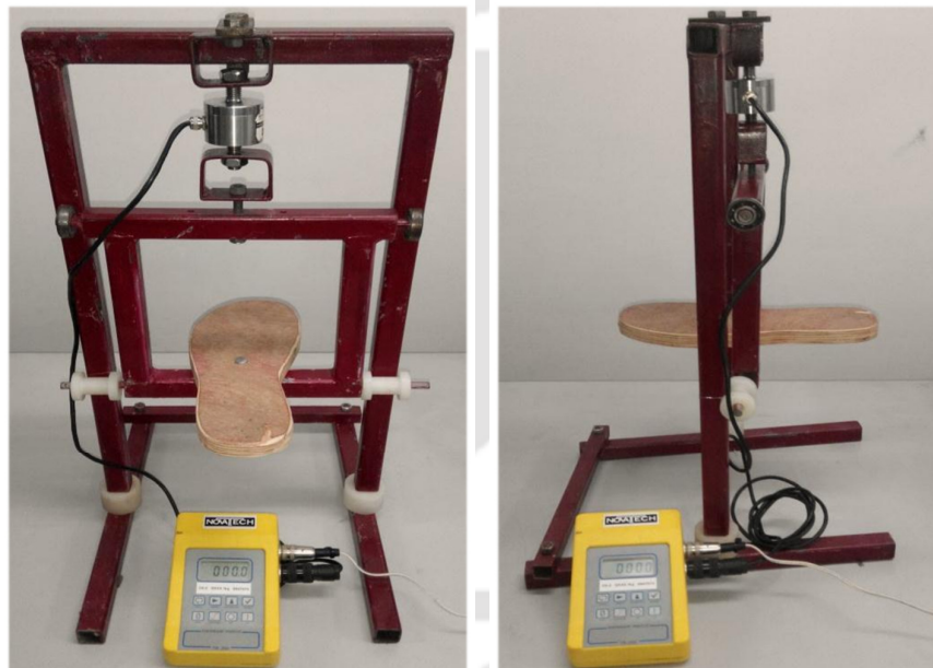
Fig. 2.11 Physical prototype of vertical isometric legs force measuring device
