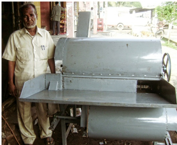
Fig. 4.2 Power operated paddy thresher invented by a farmer in Assam
