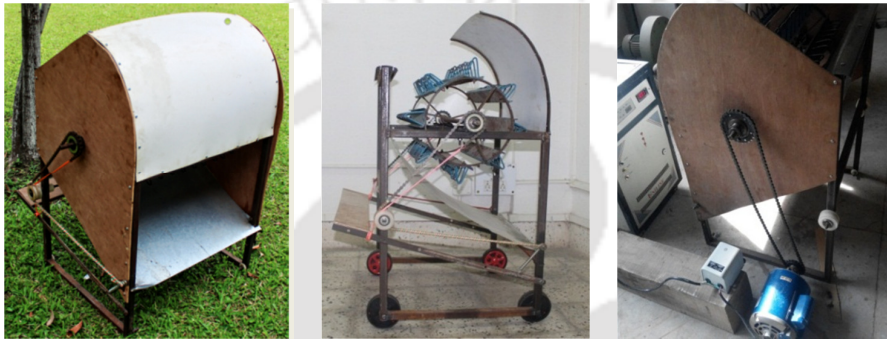
Fig. 4.20 Different views of CAD and developed prototype of pedal threshers
