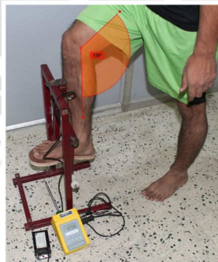
Fig. 2.1 Measurement of leg strength in standing posture at 130 o knee joint angle
