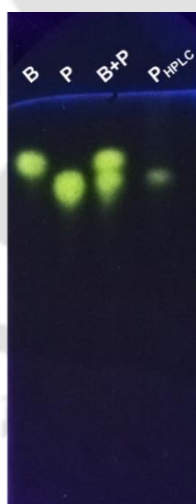
Figure 3.10: TLC analysis in solvent system of butanol: glacial acetic acid: water (14:3:4) for the confirmation of palmatine in purified HPLC eluent, where,
