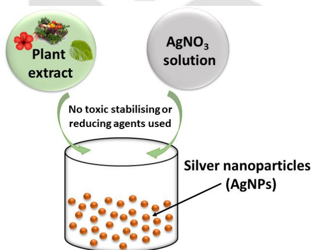
Figure 2.1. Green synthesis of silver nanoparticles using plant or agro-waste extract.
