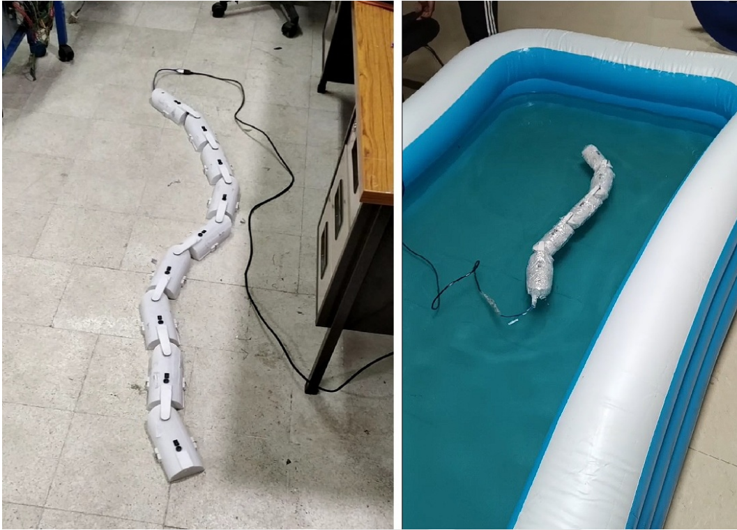
Figure 7.1: Experimental set-up of snake robot, Link1 , Link2
