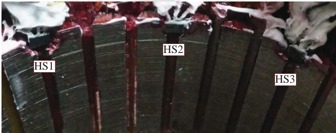
Figure 5.27: Position of Hall sensors in stator.
