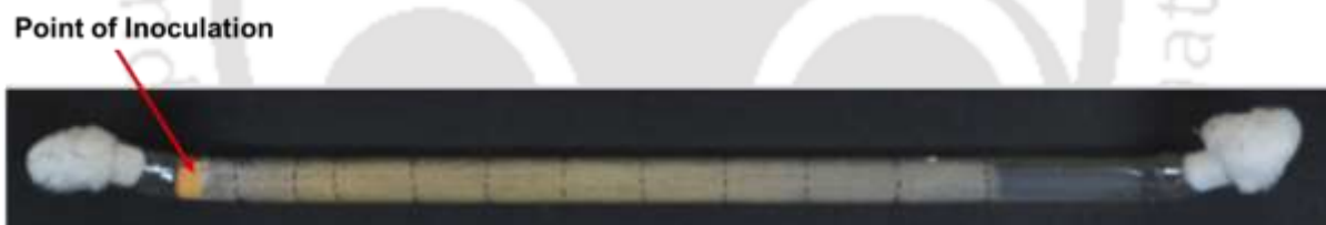
Fig. 2.5: Standard race tube assay (Top view). A race tube is hollow tube made of glass (~40 cm in length and 1.2-1.4 cm in diameter) with upward bends in both end.
