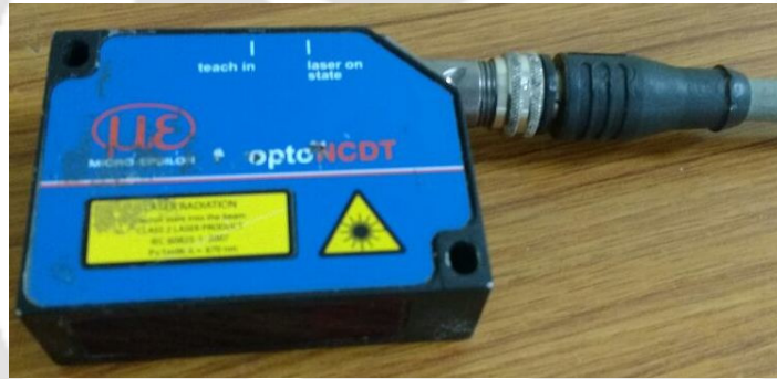
Figure 4.4: Laser displacement sensor (opto NCDT-1402-100).
