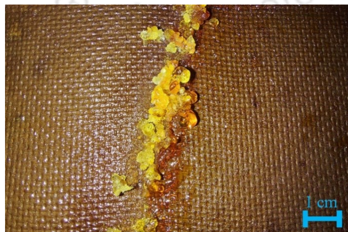
Figure 3.14: Gel balls formed on the surface of the pressboard.
