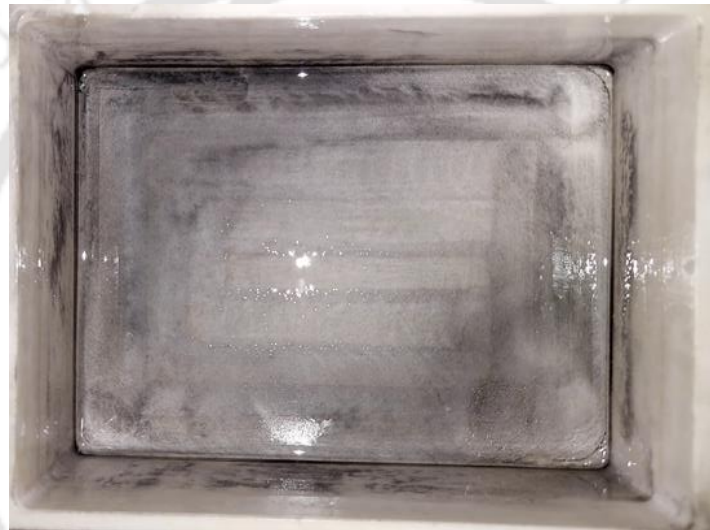
Figure 5.4: \text{Fe}_3\text{O}_4 NPs adhered to the test cell after removing the nanofluid.
