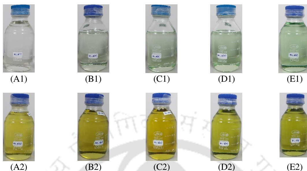
Figure 5.6: Hermetically sealed fresh and oxidative aged liquid insulation samples.
