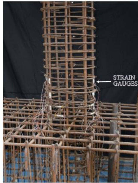
Figure 5.11. Photograph showing strain gauges fixed on rebar
