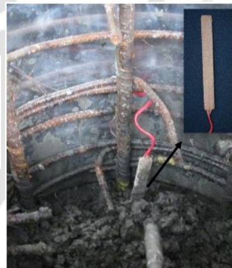
Figure 5.12. (a) Location of concrete embedded strain gauge in the specimen (b) photograph showing a sample embedded strain gauge
