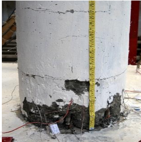
Type 3 (f) HyFRC specimens at the end of Cyclic test
