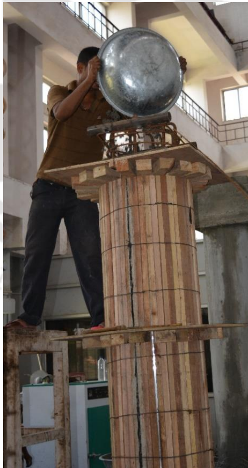
Figure 5.5. Photograph showing cast of test specimen
