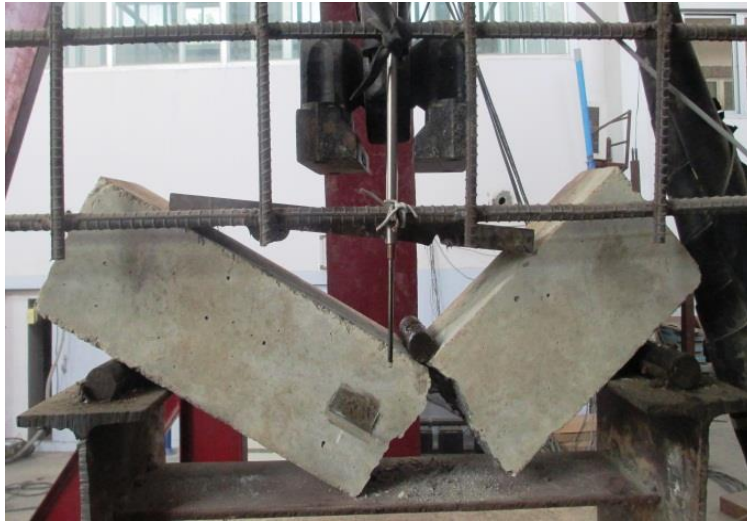
Figure 3.8. Final damaged state after testing of conventional concrete specimen
