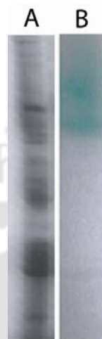
Figure 3.1: Zymogram analysis with mixed substrates namely n -heptanol, n -dodecanol, 3-octanol and benzyl alcohol. (A) CBB R-250 staining gel were recorded as B/W using Gel Documentation systems (Bio-Rad, USA). (B) Gel stained with ABTS dye to detect alcohol oxidase bands in PAGE. Photograph was recorded with CCD camera (Nikon, Japan).
