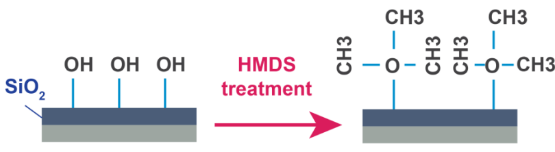
Figure 2.7 Schematic diagram of HMDS modification process on inorganic SiO 2 dielectric layer.
