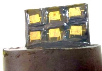
Figure 4.17: 6-device configuration sensor head: installed in Sense-city
