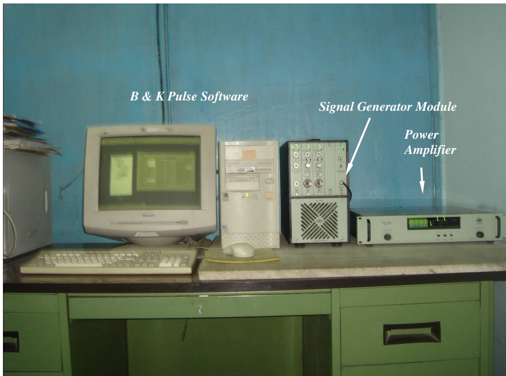
Figure 5.8 A signal generator module with a power amplifier
