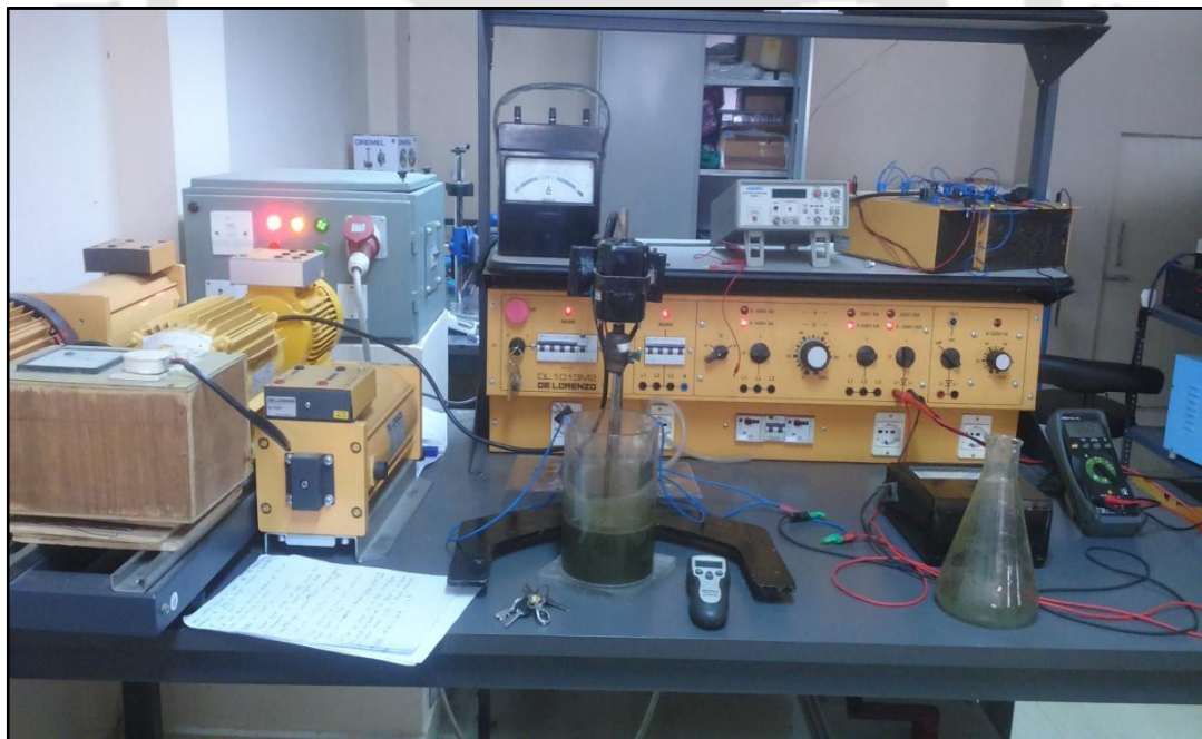
Fig. 3.6. (a) Diagrammatic representation and (b) experimental set up of electrohydrolysis pretreatment
