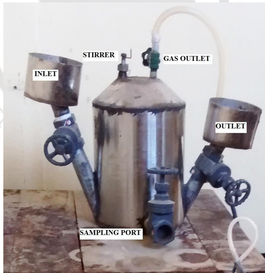
Fig. 3.9. (a) Schematic and (b) pictorial representation of the novel anaerobic digester
