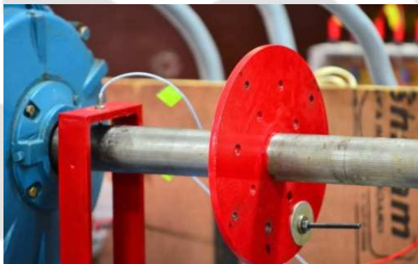
Figure 5.10: A perforated disc with known mass unbalance.
