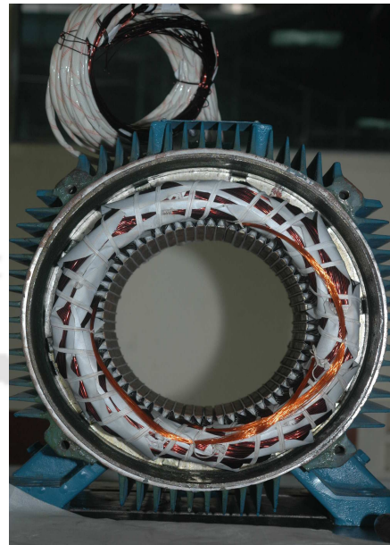
Figure 5.5: After completion of the incorporation of bridge configured winding.
