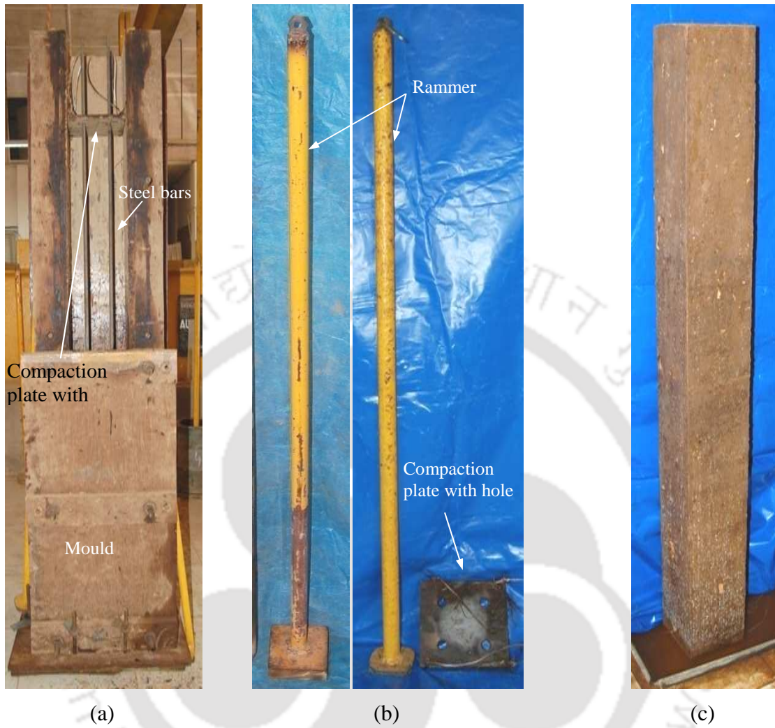
Fig. 5.3. Equipments: (a) mould; (b) rammer and compaction plate with holes; and (c) typical steel reinforced CSRE column.
