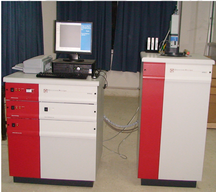
FIG. 3.13: Photographic view of a Magnetic Property Measurement System (MPMS XL 7, Quantum Design).
