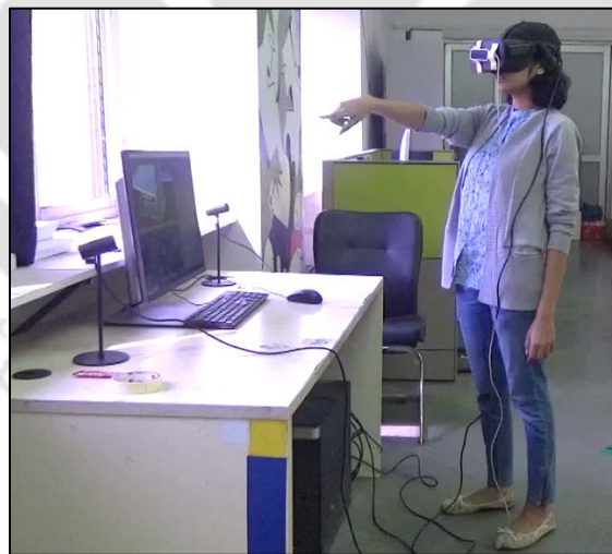
Figure 15: Experimental setup used for the study. The user is wearing Oculus Rift headset with a mounted Leap motion device. Camera placed diagonal to user took the photograph.
