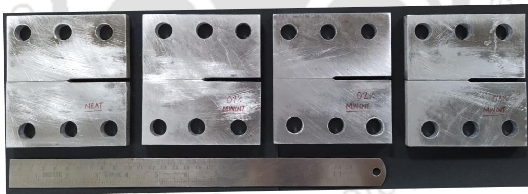
Fig. 4.9 Fabricated specimens for fracture tests (a) Pristine (b) 0.1%, (c) 0.2% and 0.3% of MWCNTs
