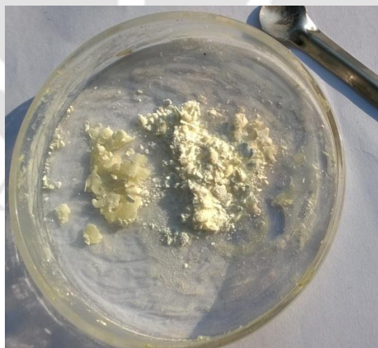
Figure 8.9 50 PEI-25K (M w = 25K) impregnated as-synthesized KIT-6
