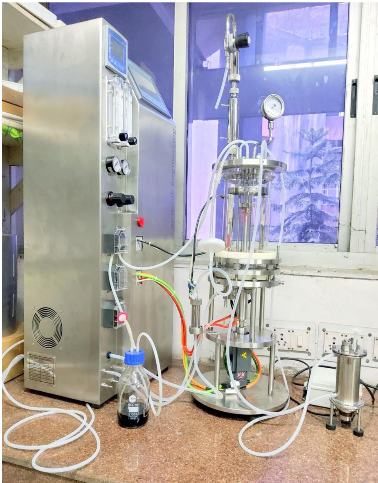
Figure S3.2: Gas fermenter setup for methane bioconversion to methanol
