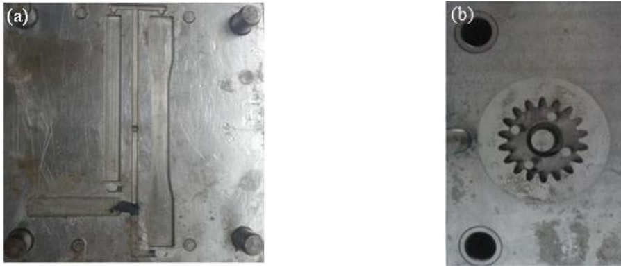
Figure 3.3 Injection molding dies for (a) tensile specimen and (b) test gear
